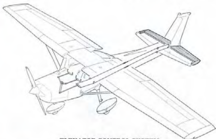
ELEVATOR CONTROL SYSTEM
